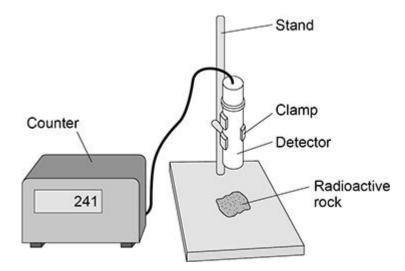
Each radioactive rock was placed below the detector one at a time.
